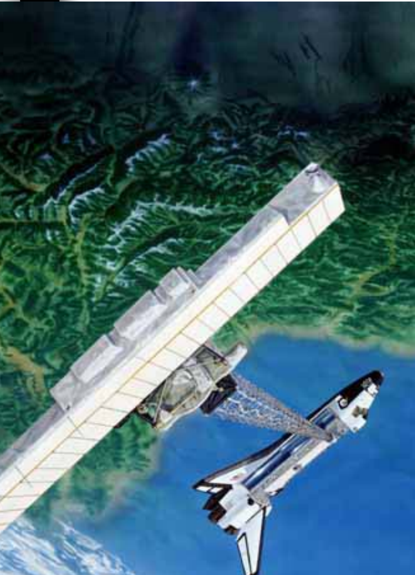
Radar signals being transmitted and received in the SRTM mission (image not to scale).
